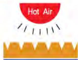
Dry the plate in hot-air dryer after taking-off the surface water with sponge roll.
